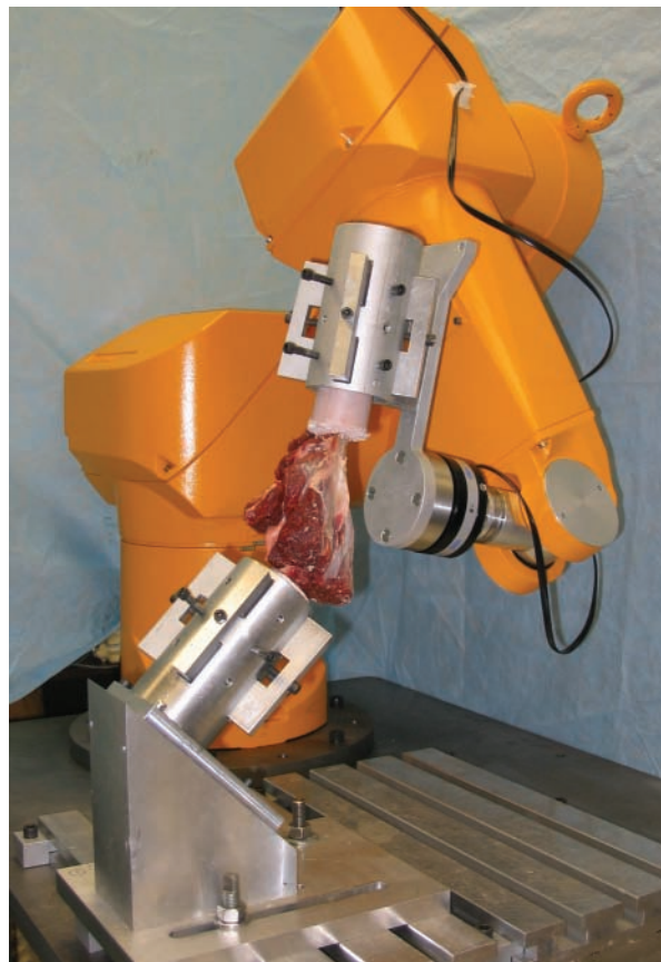
Figure 2. Test set-up of the kinematic testing using a robotic/universal force-moment sensor testing system. The tibias of the specimens were fixed to the end effector of the robot via a custom-made clamp and the femur was mounted to the base of the robot.
